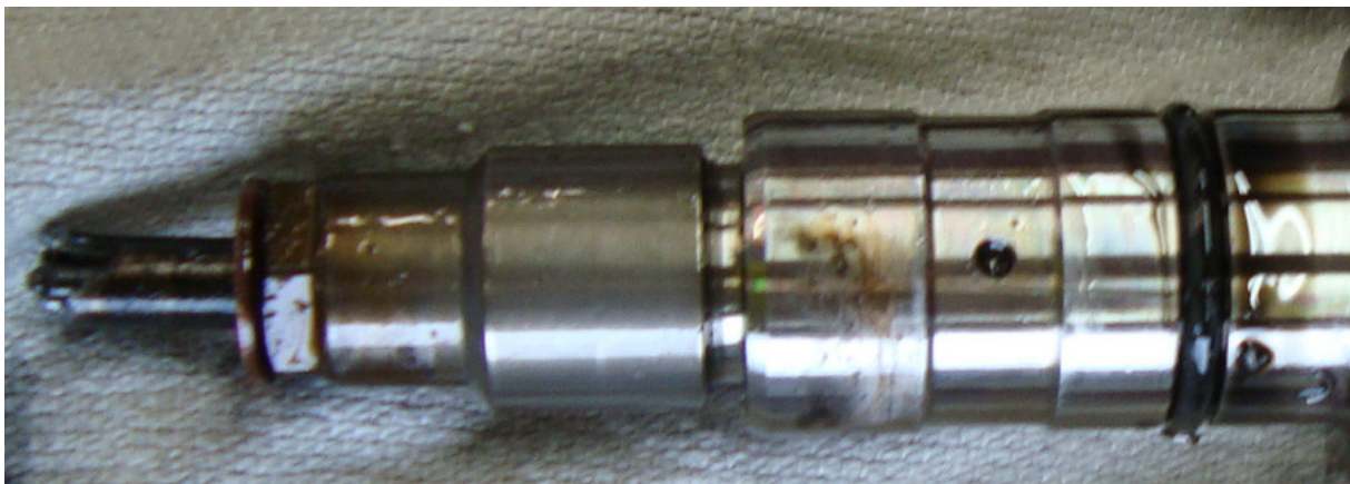
Fig. 9. Engine No. 3 – faulty injector
