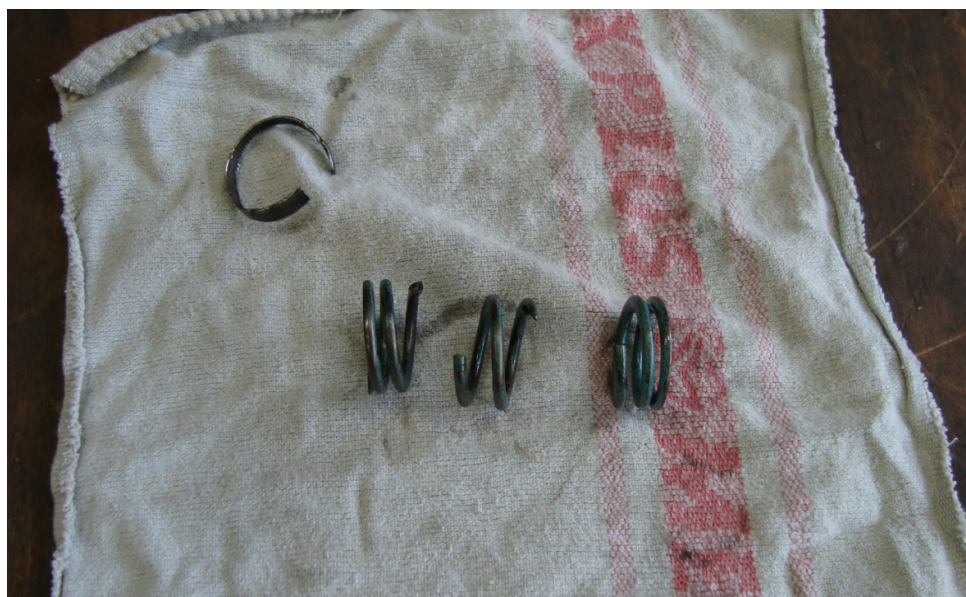
Fig. 7. Engine No. 3 – broken valve spring
