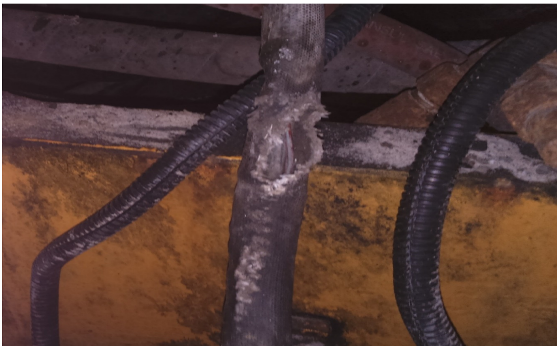
Fig. 5. Engine No. 2 – damaged loom
