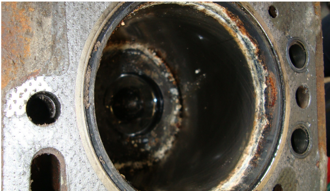
Fig. 3. Engine No. 1 – damaged number 4 cylinder sleeve and piston
