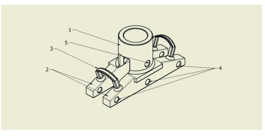
*Fig. 6. The handle is for mounting propellers wing thruster*
