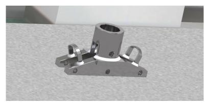
Fig. 5. Holder model for regeneration wing propellers on the universal lathe
