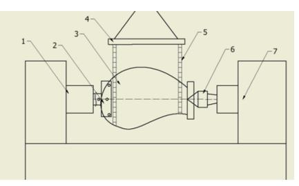
Fig. 2. Method of affixing propeller's wing in the lathe: 1. spindle, 2. handle, 3. workpiece, 4. mounting strip, 5. straps, 6. dead centre, 7. tailstock
