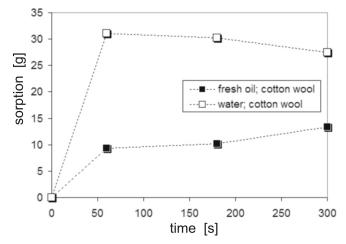
Fig. 6. Mass of absorbed oil and water as the function of the time of cotton wool contact with water
