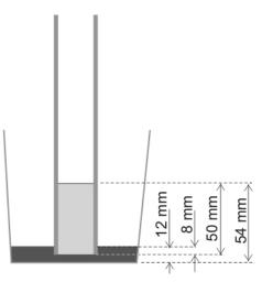
Fig. 3. Measurement geometry
