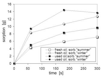
Fig. 4. Mass of absorbed oil as the function of the time of contact of the sorbent with oil
