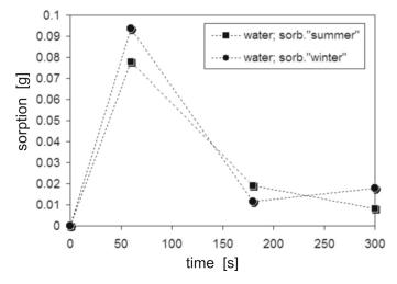
Fig. 5. Mass of absorbed water as the function of the time of contact of the sorbent with water
