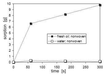
Fig. 7. Mass of absorbed oil and water as the function of time of polypropylene nonwoven contact with water
