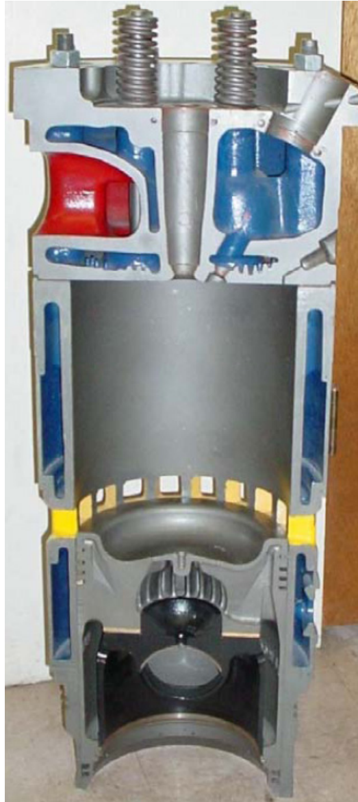
Fig. 2. EMD 645-E power assembly [2]
