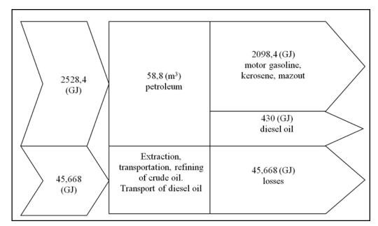
Fig. 3. The energy balance of the life cycle of diesel oil
