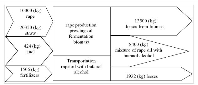
Fig. 6. The balance of the materials necessary to production 10000 litres of a mixture of rape oil and butanol alcohol (2:3 ratio)
