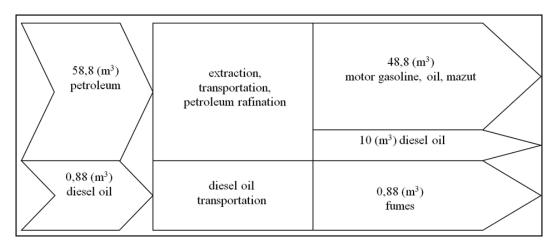
Fig. 5. The balance of raw material sourcing 10,000 litres of diesel oil
