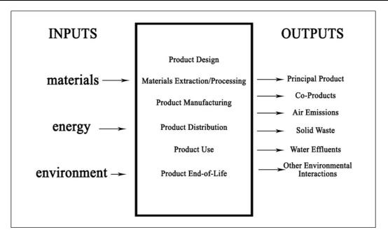
Fig. 2. Schematic structure of the LCA
