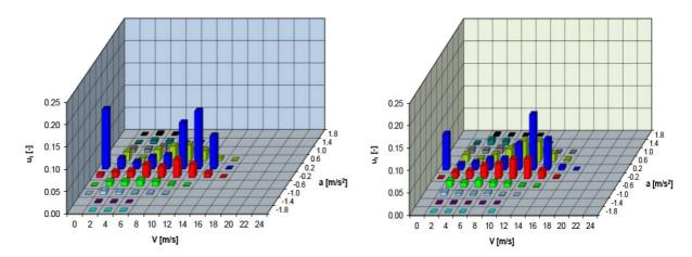
Fig. 5. Two-dimensional histograms of participation of the vehicle operation time during testing in coordinates of the vehicle speed - acceleration: - vehicle I (CNG), - vehicle II (diesel)
