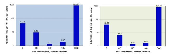
Fig. 11. Results of the road fuel consumption and the road emission of substances obtained during testing
