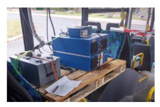
Fig. 9. Mobile device Semtech DS to measurement of exhaust emission pollutants under real conditions
