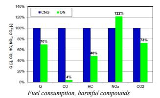
Fig. 7. Comparison of the road consumption of fuel and the road emission of pollutants, obtained during testing
