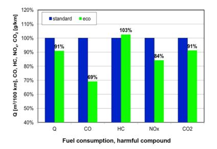
Fig. 12. Percentage changes in fuel consumption and harmful compound, tested buses
