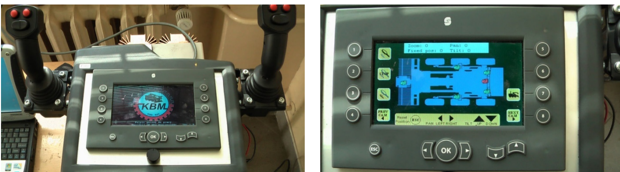
Fig. 5. The mission support engineer robot's remote control panel
