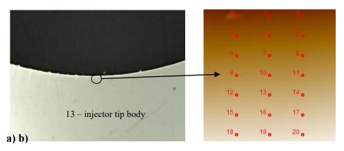
Fig. 2. The view of the investigated sample: a) an enlarged view – injector tip body (used), b) distribution of the measuring points
