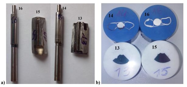
Fig. 1. The investigated parts of DLLA 160 S 1305 injector: a) the view of the injector needle and body, b) the corresponding prepared samples; 16 – new injector tip needle, 14 – used injector tip needle, 15 – new injector tip body, 13 – used injector tip body
