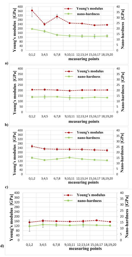
*Fig. 5. The dependence of nano-hardness and Young's modulus values on depth under the surface: a) new injector tip body, b) new injector tip needle, c) used injector tip body, d) used injector tip needle*
