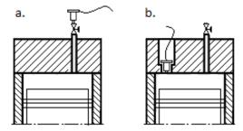
Fig. 1. The sensors for measuring the pressure of the cylinder: a) on the indicator cock, b) in a special channel cylinder head
