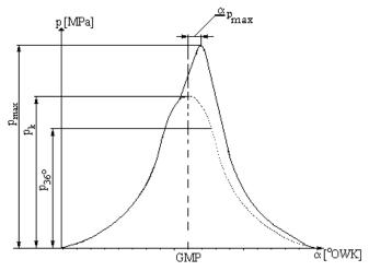
Fig. 2. Indicator diagram obtained from the electronic indicator and its characteristic values:  $p_{max}$  – the maximum combustion pressure,  $p_k$  – compression pressure,  $p_{36^\circ}$  (or  $p_{exp}$ ) – expansion pressure read 36 degrees of crankshaft rotation after TDC,  $\alpha_{pmax}$  – angle after TDC obtain maximum pressure in the cylinder
