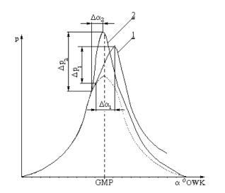
*Fig. 4. Exemplary indicator diagram (1) and diagram with high value of*  $\Delta p / \Delta \alpha$  *(2)*
