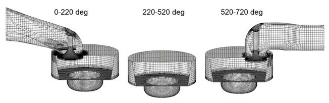
Fig. 1. The computational mesh of engine
