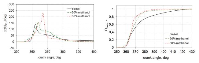
Fig. 3. Heat release rate  $(dQ/d\phi)$  and accumulative heat release (Q), (injection timing: 8.5 deg before TDC)
