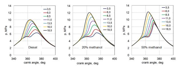
Fig. 4. The courses of the combustion pressure in a diesel and dual fuel engine
