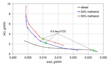
Fig. 5. The interdependence of NO and soot emission in a dual fuel engine
