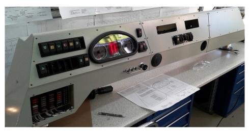
Fig. 4. The ON-13 Driver's Dashboard
