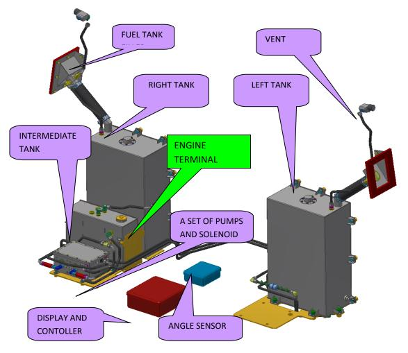
Fig. 10. Diagram of the fuel system
