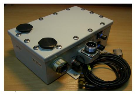
Fig. 7. Voltage Regulator RN-10U2
