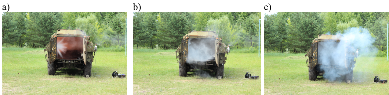
Fig. 8. Pictures of selected sequence for extinguishing standard fuel test fire leaking under pressure in the vehicle combat compartment: a – extinguishing fuel fire, b – end of standard fire extinguishing; c – smoke outflow from crew compartment after extinguishing fire
