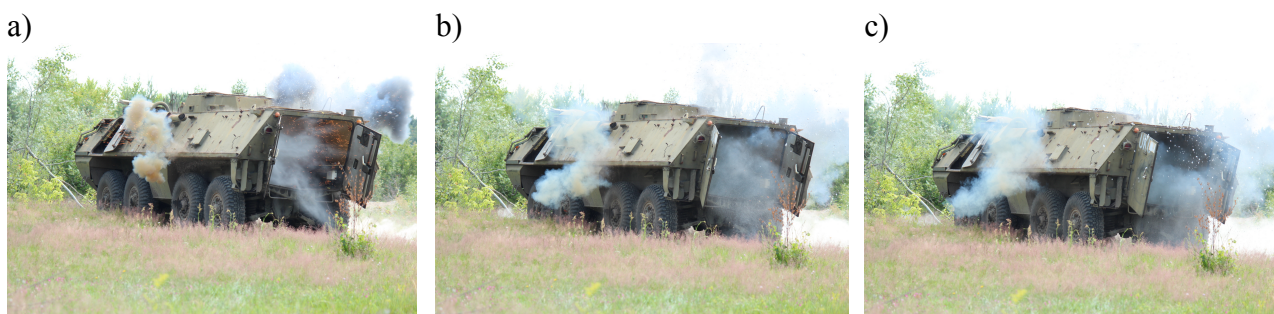
Fig. 9. The picture of selected extinguishing/suppression sequence of fuel explosion dispersed after punching of fuel container by the cumulative flow in the vehicle combat compartment: a – fuel ignition by cumulative flow; b – fuel extinguishing; c – smoke outflow from combat compartment upon fire extinguishing
