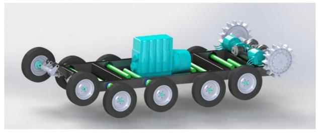
*Fig. 5. The configuration of the WIPH vehicle wheels and steering system*
