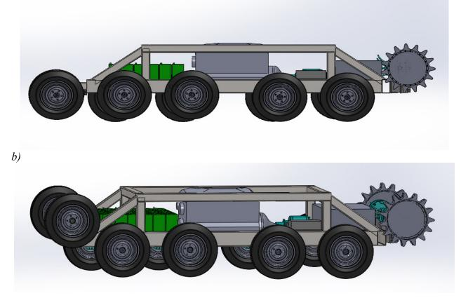
Fig. 6. Suspension configuration with a) lowered and b) raised first pair of road wheels
