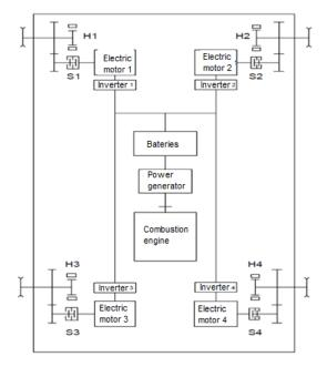
Fig. 4. Diagram of the hybrid drive concept
