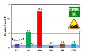
Fig. 8. Values of emission factors for a vehicle fitted with a diesel engine in Euro 5 emission class obtained in emission tests in mountainous terrain
