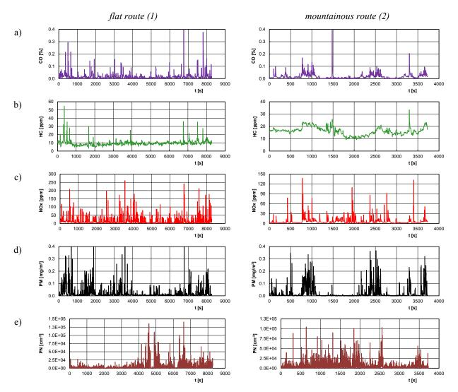
*Fig. 4.* Concentration while driving along flat route and mountainous route: a) carbon monoxide, b) hydrocarbons, c) nitrogen oxide, d) particulate mass, e) particulate number (gasoline engine)
