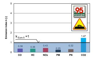
Fig. 5. Values of emission factors for a vehicle fitted with a petrol engine in Euro 5 emission class obtained in emission tests in flat terrain
