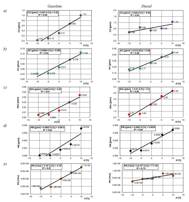
Fig. 9. The relation between the average road emission and the route grade for: a) carbon monoxide, b) hydrocarbons, c) nitrogen oxide, d) particle mass, e) particle number
