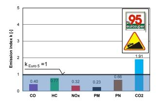
Fig. 6. Values of emission factors for a vehicle fitted with a petrol engine in Euro 5 emission class obtained in emission tests in mountainous terrain
