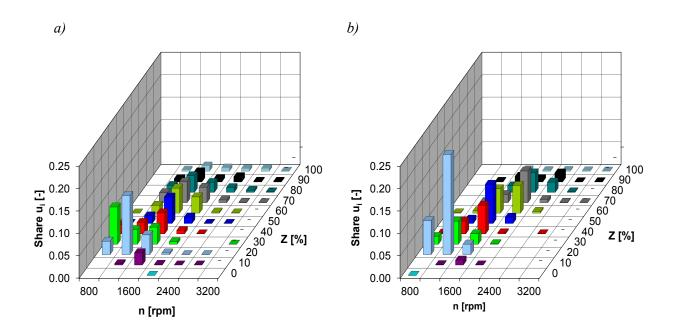
Fig. 3. Engine operational conditions against coordinates' engine speed-engine load during the road tests: a) flat route, b) mountainous area
