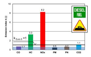
Fig. 7. Values of emission factors for a vehicle fitted with a diesel engine in Euro 5 emission class obtained in emission tests in flat terrain
