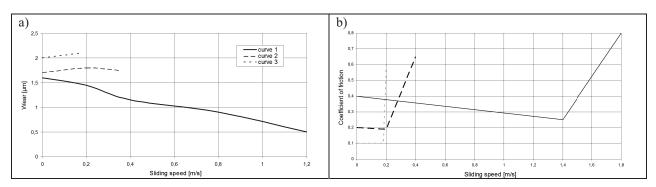
Fig. 6. Dependence of wear on the sliding speed for the matching of the friction assembly of the ball plunger face made of steel 18HNWA with the swivel disk made of steel EI-928; 1-pressure  $P_{os} = 100 \text{ N}$ , 2- pressure  $P_{os} = 600 \text{ N}$ , 3- pressure  $P_{os} = 1400 \text{ N}$
