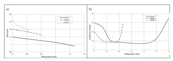
Fig. 5. Dependence of wear (a) and the coefficient of friction (b) on the sliding speed for the matching of the friction assembly of the ball plunger face made of steel 12HN3A with the swivel disk made of steel EI-928; 1-pressure  $P_{os} = 100 \text{ N}$ , 2- pressure  $P_{os} = 600 \text{ N}$ , 3- pressure  $P_{os} = 1400 \text{ N}$
