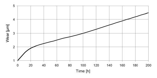
*Fig. 9. Change of the wear of the working surface of the steering swivel disk in the pump NP-34, depending on the working time (one of the result achieved during the station tests)*
