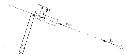
Fig. 1. Diagram of loading the hydraulic plunger assembly:  $F_{pc}$  – pressure force of the working liquid;  $F_{bezw}$  – inertial force by relative movement;  $F_{od}$  – centrifugal force; R – reaction force of the plunger face;  $F_1$  and  $F_2$  – components of the centrifugal force
