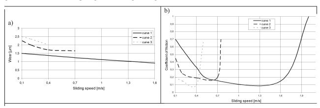
Fig. 4. Dependence of wear (a) and the coefficient of friction (b) on the sliding speed for the matching of the friction assembly of the ball plunger face made of steel HWG with the swivel disk made of steel EI-928; 1-pressure  $P_{os} = 100 N$ , 2-pressure  $P_{os} = 1400 N$ , 3-pressure  $P_{os} = 600 N$
