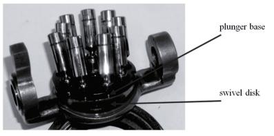
Fig. 2. Connection of the plunger base and the working surface of the swivel disk in the hydraulic plunger pump
