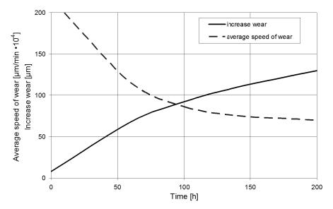
Fig. 8. Change of the wear of the ball plunger face in the pump NP-34, depending on the working time (one of the result achieved during the stand tests)
