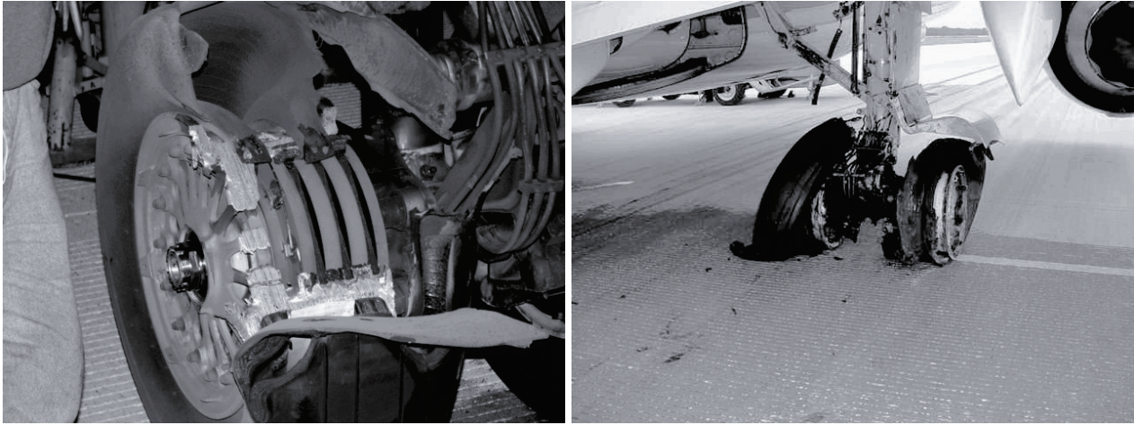
Fig. 1. Landing Gear damaged by burned tire after excessive braking [6]
