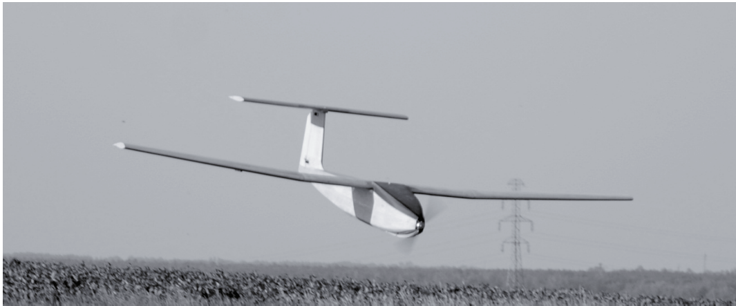
Fig. 6. Test flight of the fuel-cell powered UAV (own source)
