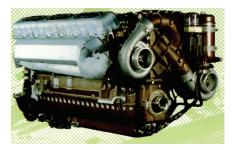
Fig. 5. Photo of the twelve-cylinder Diesel engine, for which one has developed the new composite pistons [6]
