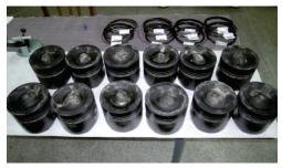
Fig. 4. Diesel engine pistons after the motor tests
