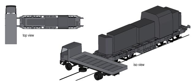
Fig. 1. FE model of the locomotive and the truck located on a level crossing - FE mesh not shown
