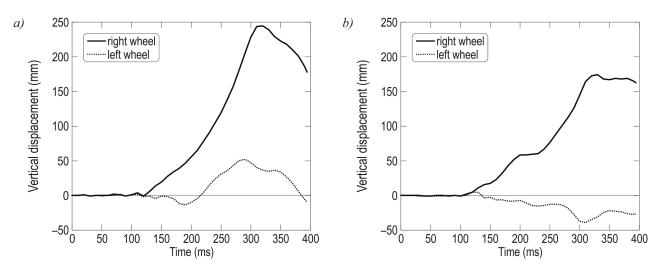
*Fig. 6. Time history of vertical displacement of the axleboxes for the first (a) and the second (b) wheelset of the front bogie confirming a serious risk of the locomotive derailment*
