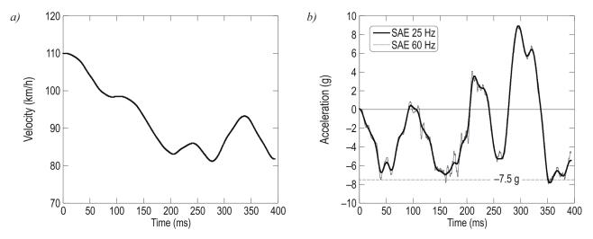
Fig. 3. Velocity (a) and acceleration (b) of the locomotive cab obtained from the FE analysis
