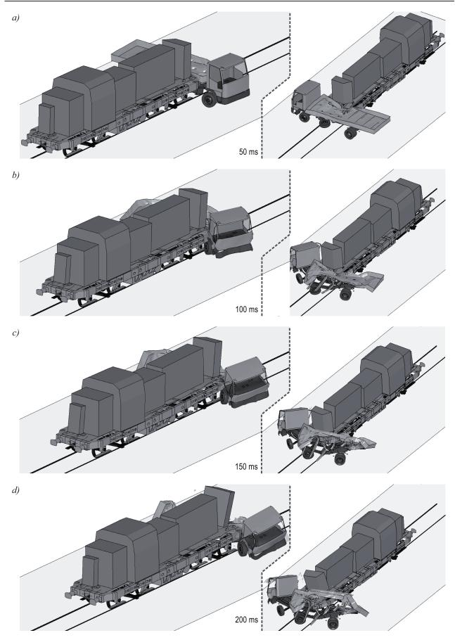
*Fig. 4. Isometric views of collision between the shunting locomotive and the 15-ton truck for selected moments of time:* 50 ms (a), 100 ms (b), 150 ms (c), 200 ms (d)
