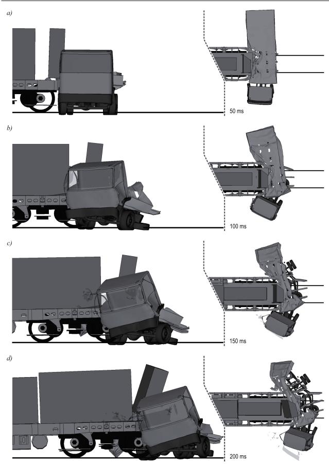
*Fig. 5. Side and top view of collision between the shunting locomotive and the 15-ton truck for selected moments of time:* 50 ms (a), 100 ms (b), 150 ms (c), 200 ms (d)
