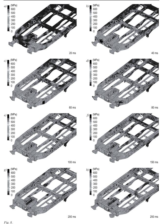
Contours of the effective von Mises stress for the locomotive frame in selected moments of time: 20 ms (a), 40 ms (b), 60 ms (c), 80 ms (d), 100 ms (e), 150 ms (f), 200 ms (g), 250 ms (h)
