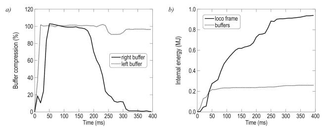
*Fig. 7. Time history of buffers' compression (a) and internal energy of buffers and the locomotive frame (b) obtained from the FE analysis*
