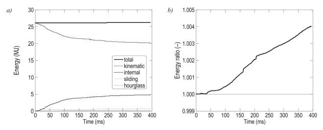
Fig. 2. Energy balance (a) and the energy ratio (b) obtained from the analysis for the complete FE model
