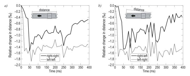
Fig. 9. Relative changes in longitudinal (a) and diagonal (b) distance between buffer attachments
