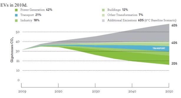
Fig. 1. Role of transport in  $CO_2$  reduction (% = 2050 estimate)
