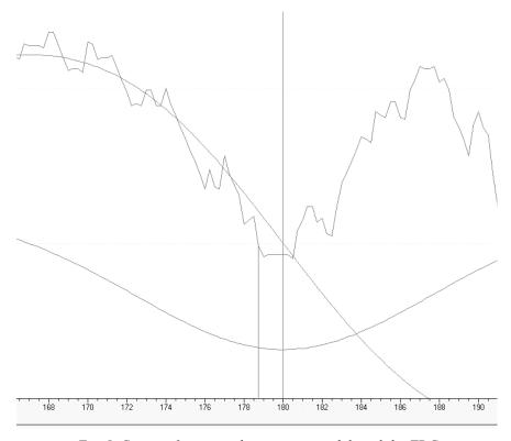
Fig. 5. Course of pressure derivative around the cylider TDC
