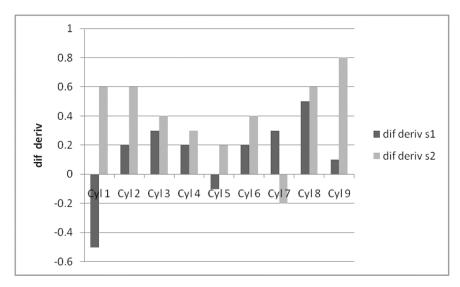
Fig. 4. Differences between designated TDC position and zero point of the first order derivative
