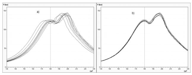
Fig. 6. Comparison of indicator graphs for all cylinder of medium speed engine MEN L32/32: a before TDC correction (directly from measurement), b after automatic TDC correction
