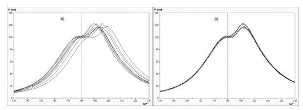
Fig. 3. Comparison of indicator graphs for all cylinder of low speed engine 9RTA96C: a before TDC correction (directly from measurement), b after TDC correction
