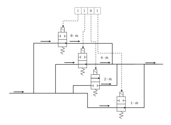
Fig. 2. The scheme and control of binary multi-valve
