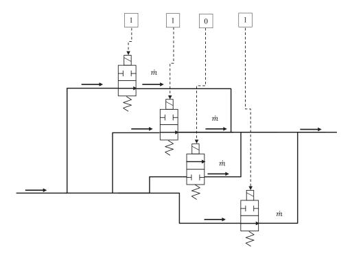
Fig. 4. The scheme and control of digital multi-valve
