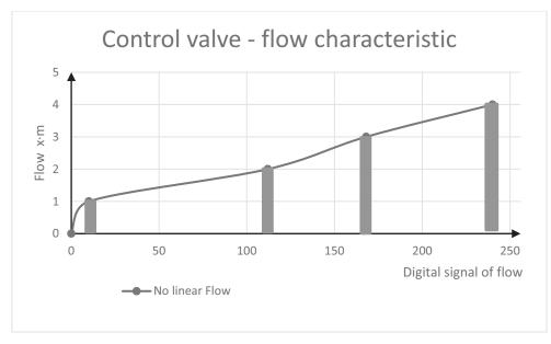
Fig. 6. The revised flow characteristics through a digital multi-valve
