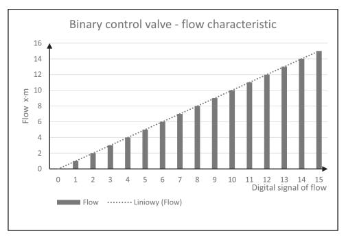
Fig. 3. Characteristics of flow through binary multi-valve
