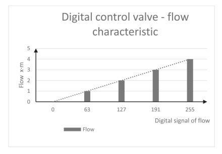
Fig. 5. Characteristics of flow through digital multi-valve
