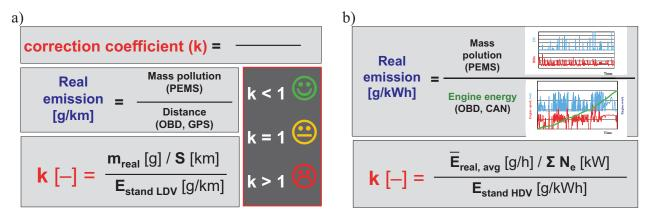
Fig. 11. Definition of correction coefficient: a) for passenger cars, b) for heavy-duty vehicle
