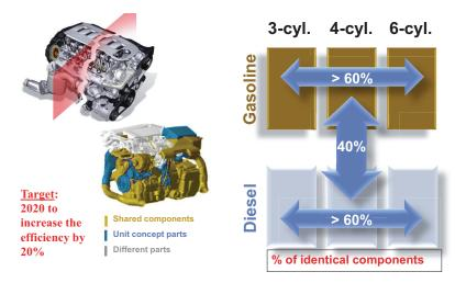
Fig. 7. The similarities between Diesel and Gasoline engines by BMW [7]
