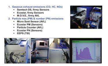
Fig. 9. Exhaust emissions measurement equipment
