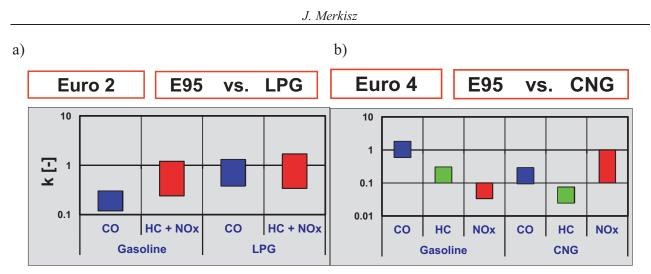
Fig. 13. Comparison of the exhaust emissions from vehicles: a) fuelled with gasoline and LPG (spark ignition engines), b) fuelled with gasoline and CNG (spark ignition engines)
