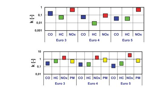
*Fig. 12. Comparison of the vehicle exhausts emissions using different vehicle emission categories: a) gasoline engine, b) diesel engine*
