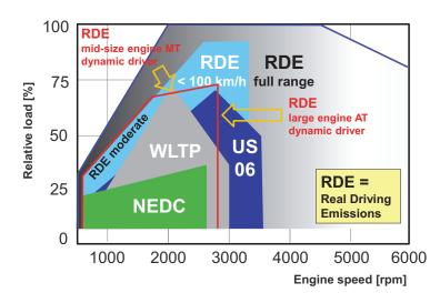
Fig. 10. Engine operating parameters in various emissions tests [16]
