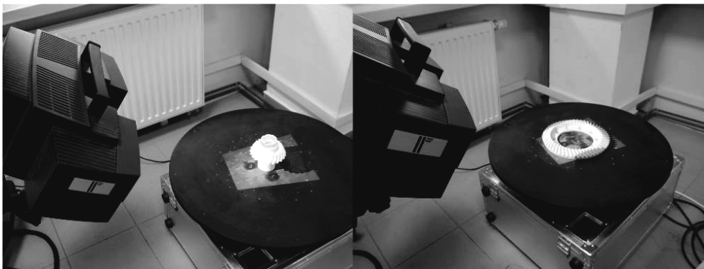
Fig. 3. Measuring of bevel gears conducted in particular positions on measuring table with the use of optical scanner 3D ATOS II Triple Scan
