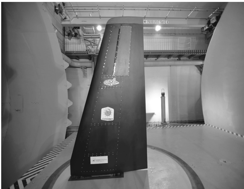
Fig. 4. The semi-span wing in the wind tunnel T-3
