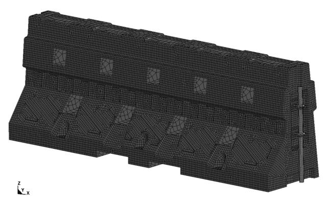
Fig. 4. A view of a non-deformable barrier with reinforcement bars and a bolt
