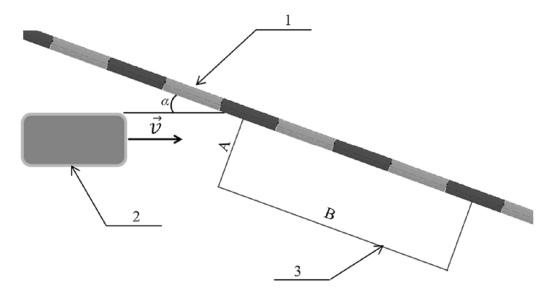
Fig. 6. A diagram of a test track used for simulation tests – collision of vehicles with a rigid or deformable safety barrier, according to PN-EN 1317-2, where: 1 - segment safety barrier; 2 - test vehicle; 3 - acceptable test car reflection field (A - width, B - length, measured in [m]); v - impact speed [km/h];  $\alpha - impact$  angle in degrees
