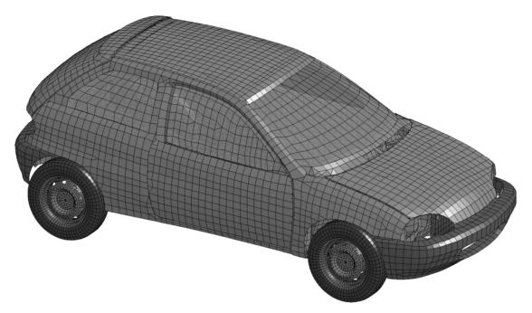
Fig. 3. Numerical model of the Geo Metro car [8]
