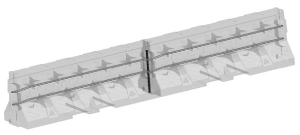
Fig.2. Safety barrier segment connecting method
