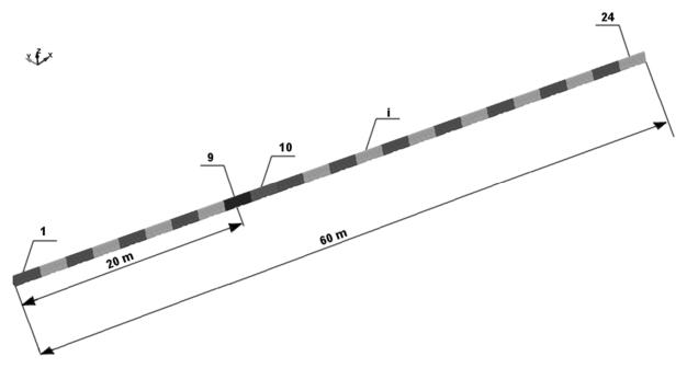
Fig. 5. Barrier configuration using two deformable segments (9 and 10): i – segment number
