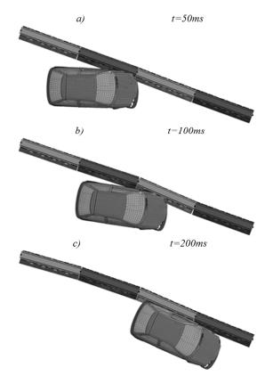
Fig. 7. Stages of a collision of the car and the barrier: a) for t = 50 ms, b) for t = 100 ms, c) for t = 200 ms
