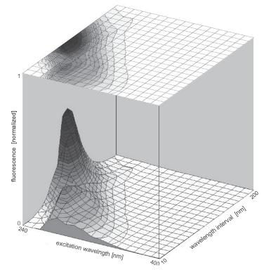
Fig. 1. Example of the total synchronous fluorescence spectra of oil (main picture) and 2D map (on the top)
