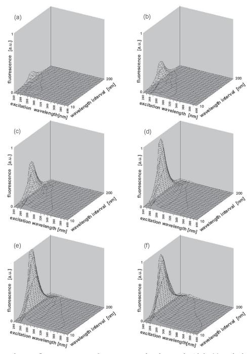
Fig. 2. Total synchronous fluorescence spectra for constant wavelength interval – Δλ for Marinol oil in n-hexane for various concentration, respectively: (a) 18 mg/kg, (b) 40 mg/kg, (c) 82 mg/kg, (d) 180 mg/kg, (e) 345 mg/kg, (f) 680 mg/kg
