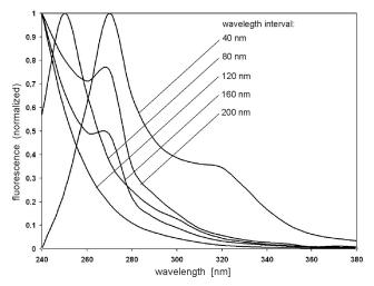
Fig. 3. Synchronous fluorescence spectra for Marinol oil in n-hexane for oil concentration 82 mg/kg normalized to the maximum value for various wavelength intervals
