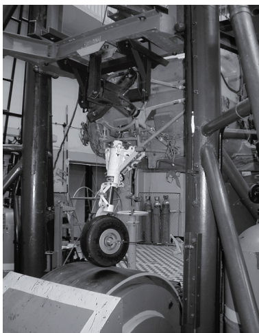
Fig. 4. M3T test stand for full scale brake testing with mounted airplane landing gear (source: IoA)
