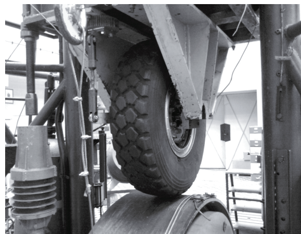
Fig. 5. M3T test stand with automotive brake and wheel mounted during tests. (source: IoA)
