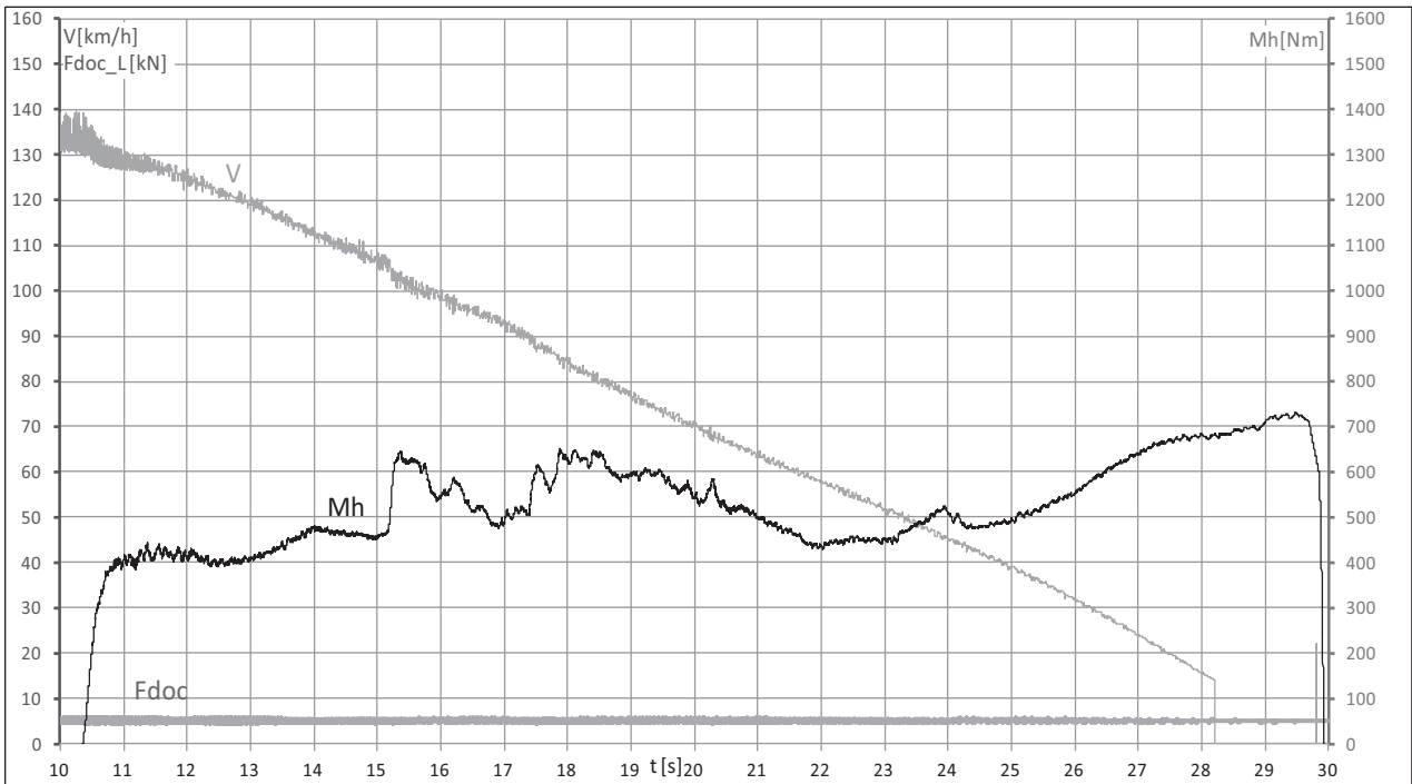
Fig. 7. Test 221, ABS-off, non-slippery surface, pushing force 5 kN
