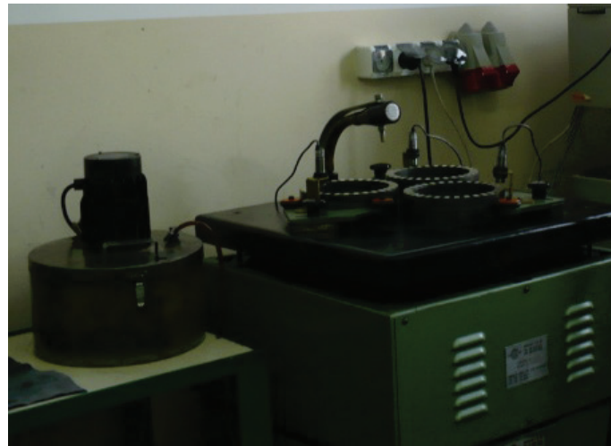
Fig. 4. One-plate lapping machine ABRALAP 380
