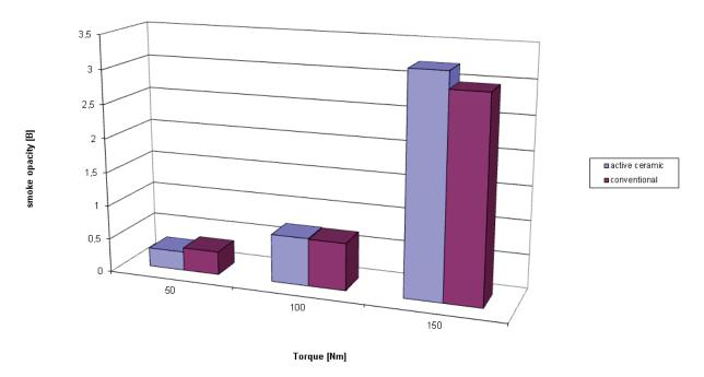
Fig. 7. Effect of load and types of valves on the degree of smoke opacity for VW 1.9 TDI at a speed of 1500 rpm
