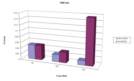
Fig. 1. Influence of load and types of valves on the CO content in the exhaust gas for VW 1.9 TDI at a speed of 1500 rpm
