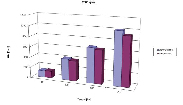
Fig. 5. Effect of load and types of valves on the content of NOx in the exhaust gas for VW 1.9 TDI at a speed of 2000 rpm
