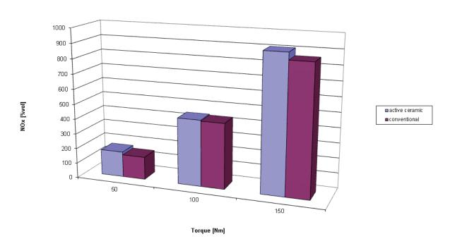
Fig. 4. Influence of load and types of valves on the content of NOx in the exhaust gas for VW 1.9 TDI at a speed of 1500 rpm
