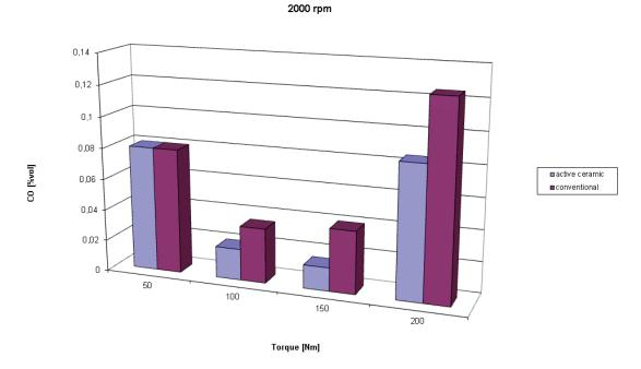
Fig. 2. Influence of load and types of valves on the CO content in the exhaust gas for VW 1.9 TDI at a speed of 2000 rpm
