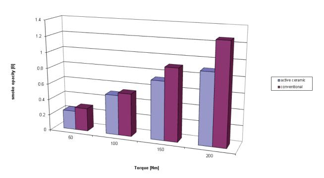
Fig. 9. Influence of load and types of valves on the degree of smoke opacity for VW 1.9 TDI at a speed of 2500 rpm
