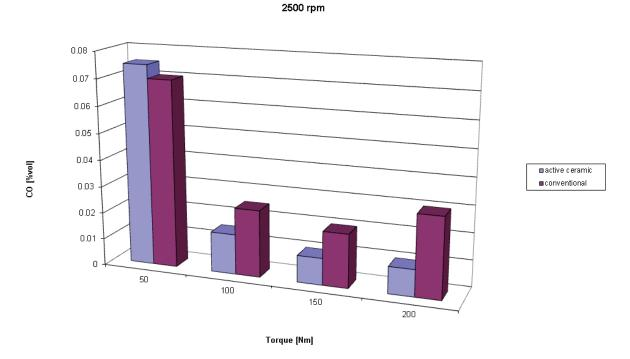
Fig. 3. Influence of load and types of valves on the CO content in the exhaust gas for VW 1.9 TDI at a speed of 2500 rpm
