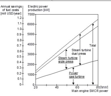
Fig. 7. Production of electric power and annual fuel costs savings of the Thermo Efficiency System as a dependency on ship main engine power [4]. Normal service: 85% SMCR, service time 280 days/year, fuel consumption: 170 g/kWh, fuel price: 160 USD/t
