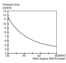
Fig. 8. Time of Thermo Efficiency System investment payback as a dependency on ship main engine power [4]. Normal service: 85% SMCR, service time 280 days/year, fuel consumption: 170 g/kWh
