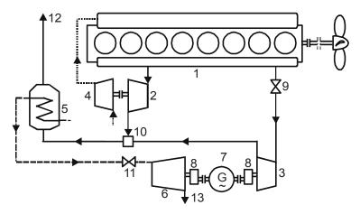
Fig. 1. Thermo Efficiency System: 1 – main engine; 2 – turbocharger turbine; 3 – power turbine; 4 – scavenging air compressor; 5 – waste heat boiler; 6 – steam turbine; 7 – generator; 8 – clutch; 9 – by-pass valve; 10 – mixing chamber; 11 – throttle valve; 12 – exhaust pipe; 13 – steam outlet
