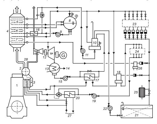
Fig. 6. Deep utilisation system utilising exhaust gases and scavenging air cooling heat: 1 – main engine;
