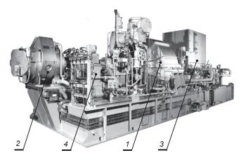
Fig. 3. Turbine generator set ABB type PTL: 1 – steam turbine; 2 – gas turbine; 3 – generator; 4 – reduction gear
