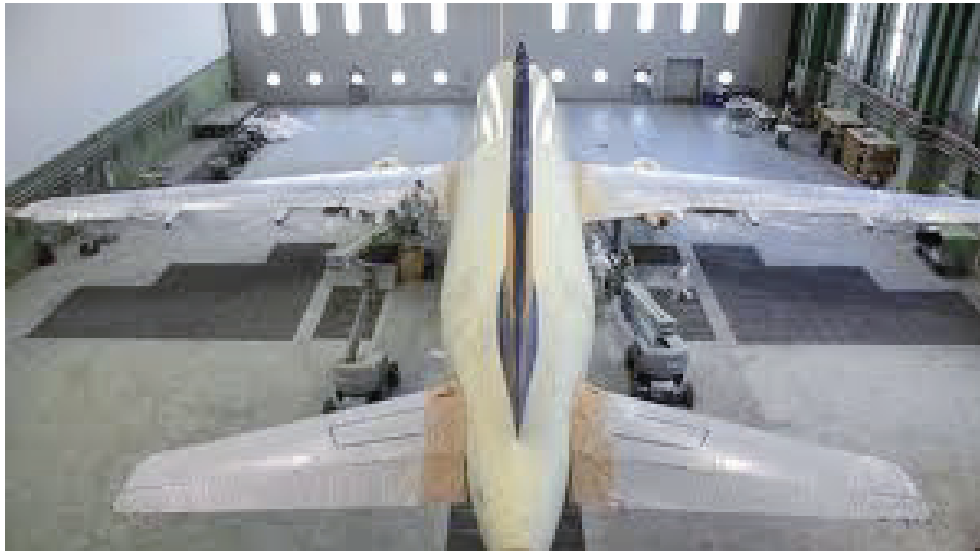
Fig. 5. Aircraft partially covered with polyurethane paint. Source vimeo.com
