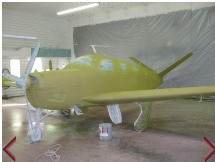
Fig. 4. Aircraft covered with etching primer Source: http://www.desapi.com
