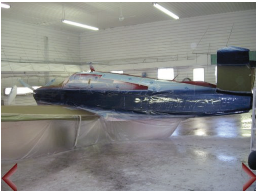
Fig. 6. Aircraft covered with colour enamel. Source: http://www.desapi.com
