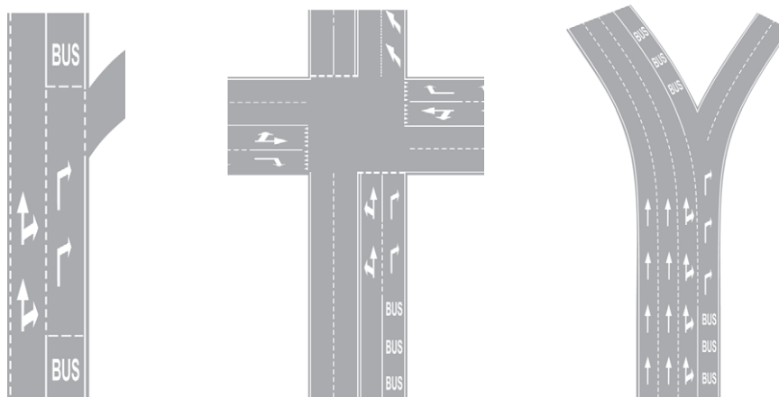
Fig. 1. Types of exclusion sections on bus lanes – from left: the section made before a non-collision turn, section before the four-inlet crossing, section designed for a road with increased speed limit
