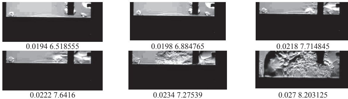
Fig. 4. Combustion course in combustion system with semi-open combustion chamber registered using digital Photram SA1.1 camera: V_P = 28\% ; CR 6:1 ; IT=50^\circ CA BTDC
