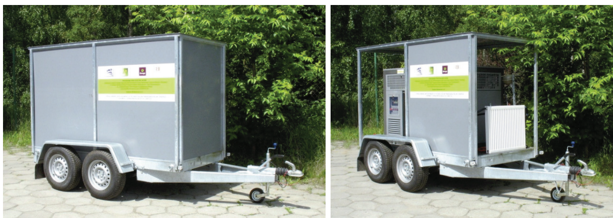
Fig. 1. Mobile unit for heat and power cogeneration on the left – fully enclosed for transport; on the right – with uncovered access to the control panel and to the gas (feed), power and heat (outlet) connections
