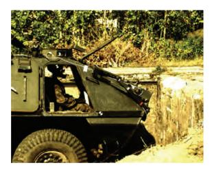
Fig. 1. The view of a test track with a rigid retaining wall and a personnel carrier prepared for a crash test
