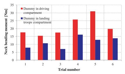
Fig. 9. The maximum values of neck bending moment
