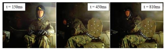
Fig. 7. Phases of motion of the dummy located in the landing troop compartment (trial no. 4)
