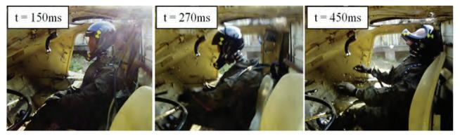
Fig. 6. Phases of motion of the dummy located in the driver's compartment (trial no. 4)
