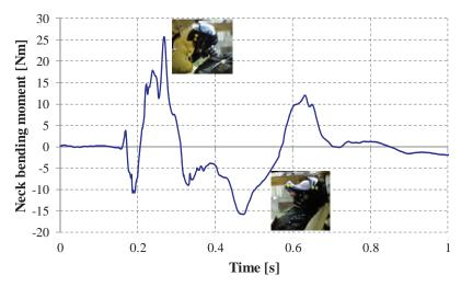
Fig. 8. The course of the neck bending moment for a dummy located in the driver's compartment (trial no. 4)
