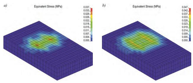
Fig. 8. Contours of the equivalent stress in the embankment under single axle (a) and 2-axle bogie (b)
