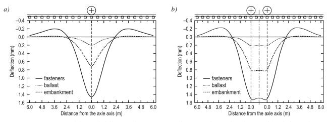
Fig. 5. Components of the track deflection along successive sleepers under single axle (a) and 2-axle bogie (b)
