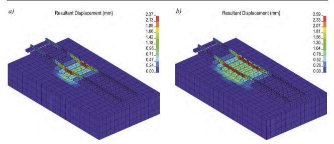
*Fig. 7. Contours of the resultant displacement in the track under single axle (a) and 2-axle bogie (b)*
