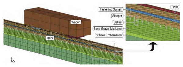
Fig. 2. FE model of the test track and wagon used in LS-DYNA dynamic analysis [4]
