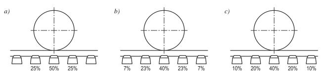
Fig. 1. Load distribution along successive sleepers: suggested by Awoleye (a), Watanabe (b), and the US Army Corps of Engineers (c) [1–3]
