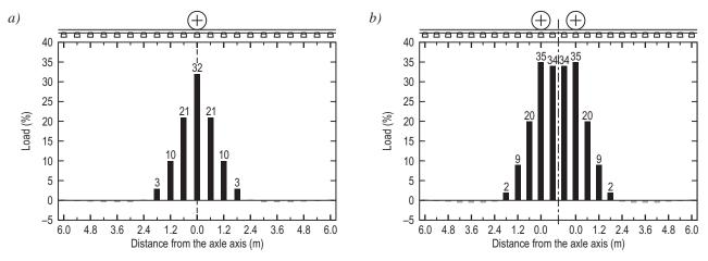
Fig. 6. Distribution of the load along successive sleepers under single axle (a) and 2-axle bogie (b)
