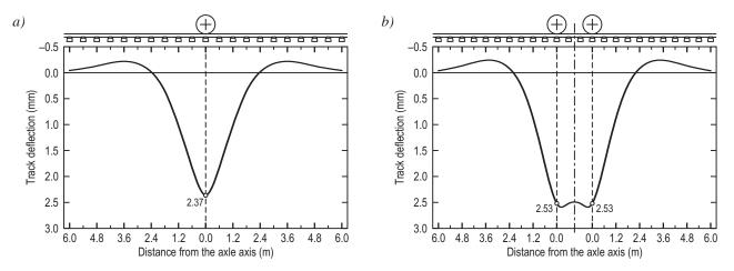
Fig. 4. Total deflection of the track along successive sleepers under single axle (a) and 2-axle bogie (b)
