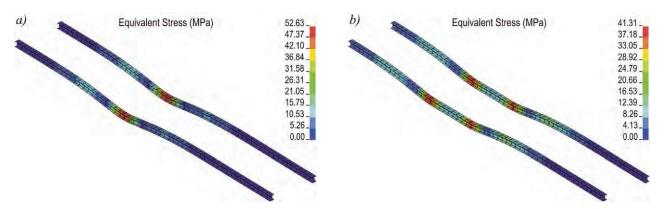
Fig. 9. Contours of the equivalent stress in rails under single axle (a) and 2-axle bogie (b)
