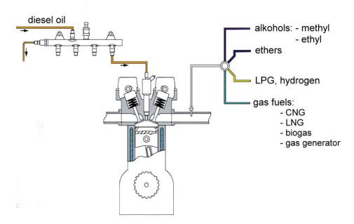
Fig. 1. Possibilities of dual fuel supply of compression ignition engine
