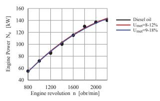
Fig. 4. Comparison of maximal power output of the SW 680 engine run in dual fuel system – fuelled with Diesel oil and methanol
