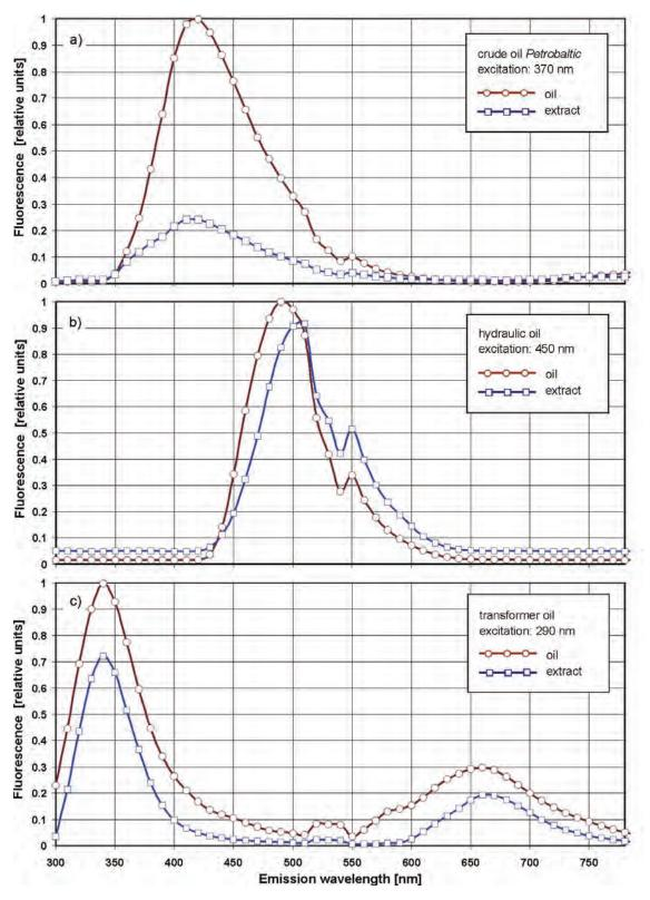
Fig. 3. Emission spectra for various excitation wavelengths for three kinds of oils and their extracts of oil-in-water emulsion
