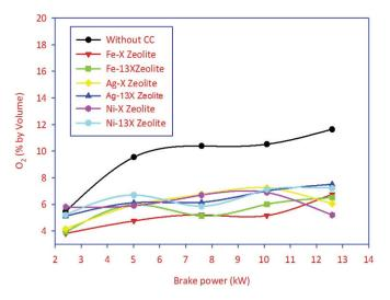
Fig.7 Oxygen against brake power
