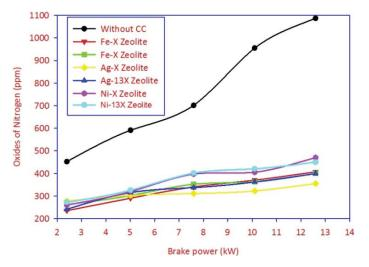
Fig. 3. Oxides of nitrogen against brake power
