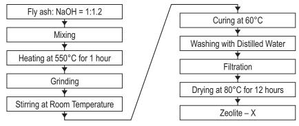
Fig. 1. Synthesis process
