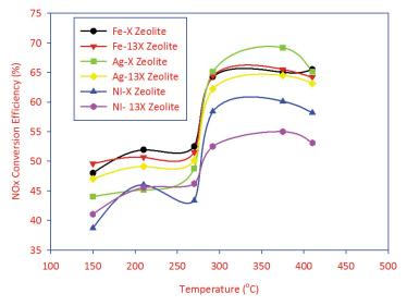
Fig. 4. NO<sub>x</sub> Conversion as a function of temperature
