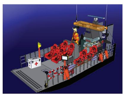
Fig. 1. One of the concepts of swimming flat-bottomed evacuation platform (Own develop of Automotive Industry Institute)
