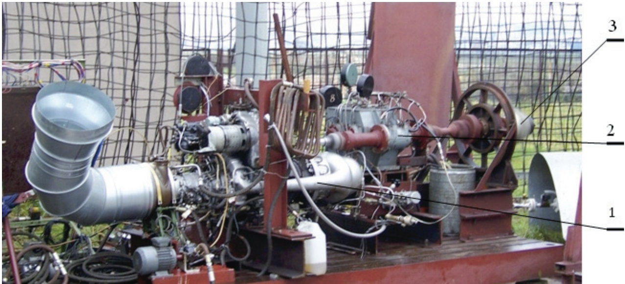
Fig. 1. View of test bench: 1 – GTD-350 engine, 2 – gear, 3 – propeller
