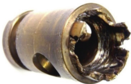
Fig. 7. View of damaged bearing
