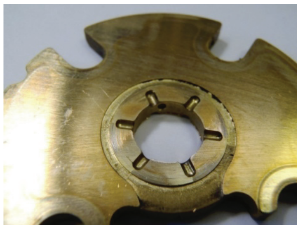
Fig. 3. View of scraped surface of bearing
