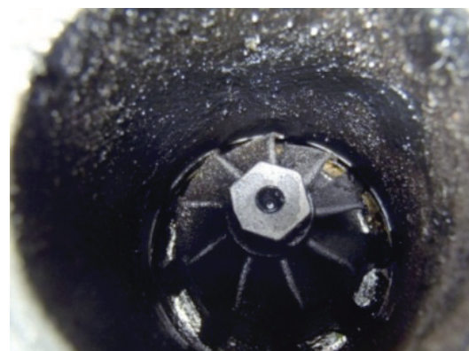
Fig. 10. View of turbine rotor with carbon depositing
