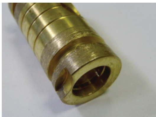
Fig. 9. View of faded bearing (dry friction)
