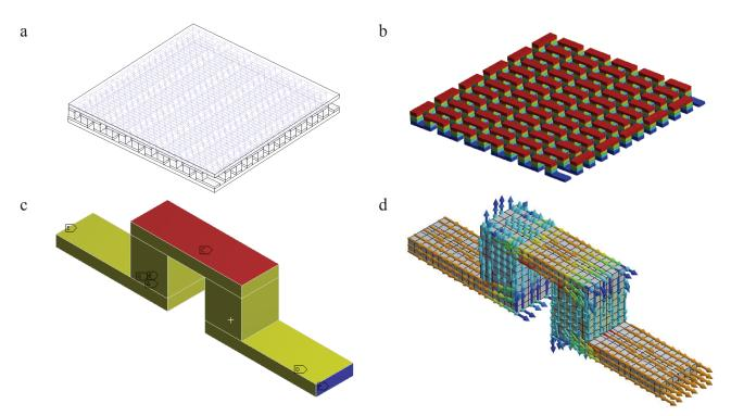
Fig. 5. Photographs of the computer TEG simulation: photograph of the TEG model, color photograph of temperature distribution, photograph of a single connector, photograph of the current flow through the connector
