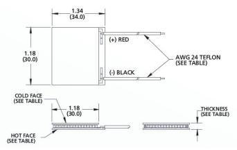
Fig. 1 Dimensions of Peltier module HT4, 12 [10]
