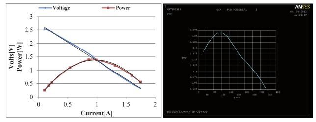
Fig. 6. load characteristics of a single TEG: a) the characteristic resulting from TEG research, b) photograph of the characteristics resulting from the computer simulation
