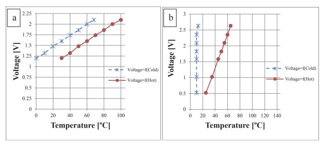
Fig. 4. Parameters of the surveyed TEG: a) for a constant temperature difference between the cold and hot side,  $\Delta T=30^{\circ}$ C, b) for a constant temperature of the cold side Tc=10°C and an increasing temperature of the hot side
