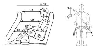
*Fig. 3. Dummy's position against cabin interior and safety belt location; BC – shoulder section of a safety belt; CE – hip section, ABCD – belt length from a retractor (A) to a lower fixing point (E). Drawings according to [5]*
