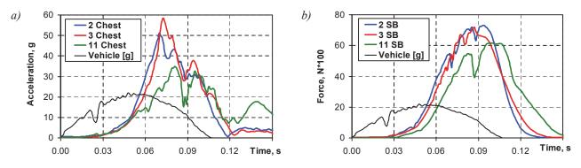
Fig. 8. Courses of torso acceleration (a) and forces (reactions) in the shoulder section of the seat belt (b)
