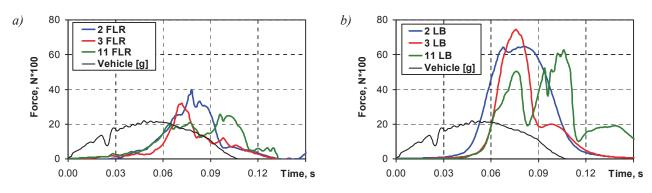
Fig.6. A course of forces in thighs (FLR) and reactions in the lap belt (LB) in the time function
