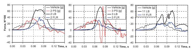
Fig. 7. Association of forces in the belts and legs with the seat back acceleration in 2P, 3P and 11P tests ("Vehicle" – body floor acceleration, PS – front seat back acceleration, LB – force in the lap belt section, FLR – a sum of forces in the left and the right legs)
