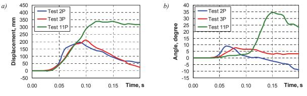
Fig. 4. Thigh longitudinal displacement (a) and thigh inclination angle (b) in 2P, 3P and 11P tests
