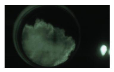
*Fig. 2. Graphic detailing a standard image captured during combustion. The bore is evident from the 'halo' of light around it with the propagating flame clear in the centre. The burst of light on the right-hand side is to indicate TDC*
