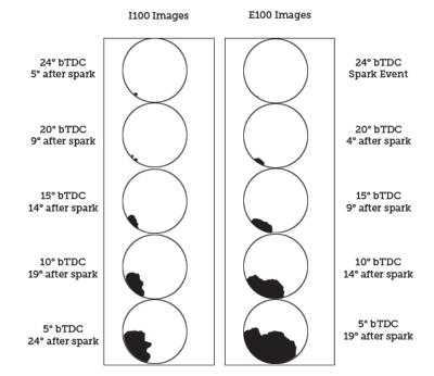
Fig. 5. Side-by-side comparison of the iso-octane (I100) and ethanol (E100) images captured
