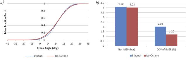
Fig. 4. a) Wiebe function curve and b) IMEP and COV of IMEP
