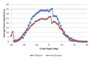
Fig. 6. Flame speed traces for both ethanol and iso-octane fuels
