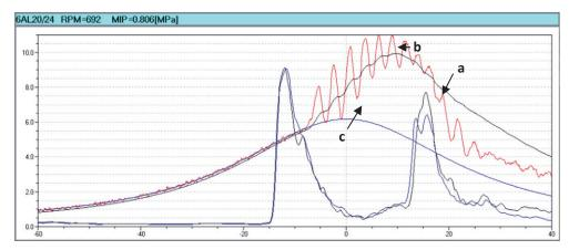
Fig. 7. Result of reconstruction of the course which has undergone filtration: a - pressure curve measured without throttling, b - the pressure curve after the reconstruction of the choked course, c - extrapolation of the compression process from the reconstructed course
