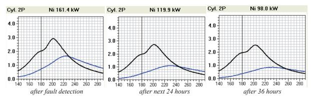
Fig. 1. Image of cylinder pressure deformed graph on the cylinder with carbon deposits in the indicating channel on the background of the average pressure graph of remaining cylinders
