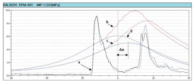
Fig. 3. An example of an indicator diagram with channel choking on a graph without choking and the TDC set by reference mark: a- the vibration pulse from the opening of the injector, b-pressure course without throttling, c-pressure course with throttling, d-extrapolations of compression curves,  $\Delta a$ - TDC shift induced by throttling
