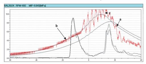
Fig. 6. An example of the pressure curve reconstruction: a – pressure curve measured without throttling, b - pressure curve measured with throttling of the channel, c - b pressure curve after reconstruction
