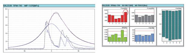
Fig. 10. The result of parameters adjustment with the assumption that throttling occur in the indicating channel cylinder no. 6
