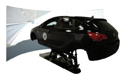
Fig. 2. AutoSim AS 1200-6 advanced high-class car simulator
