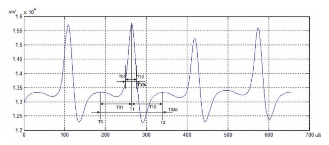
Fig. 2. Signal from induction sensor
