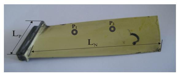
Fig. 1. First grade blade of axial compressor of aircraft engine SO-3  $L_N$ =113 mm,  $L_p$ =40 mm with indicated points of oscillation inductor
