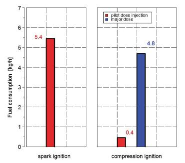
*Fig. 4. Comparison of the fuel consumption the test engine working in spark ignition and compression ignition mode for the speed 2500 rpm*
