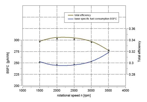
*Fig. 3. Course of specific fuel consumption and total efficiency as a function of crank angle for the test engine working with spark ignition mode*
