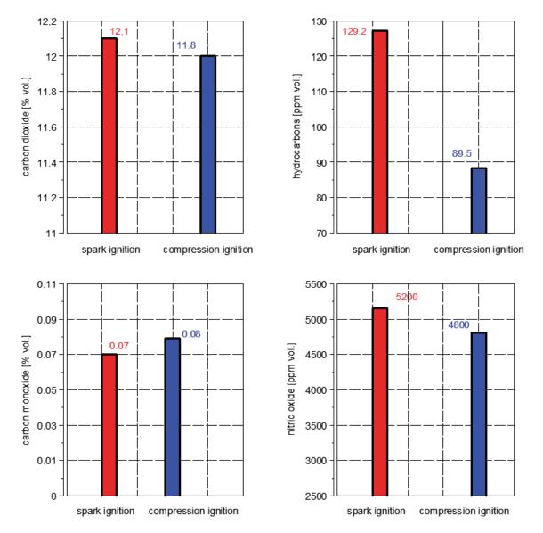
Figure 7 shows the content of toxic gases, namely, carbon dioxide, carbon monoxide, nitrogen oxide and hydrocarbons for engine working with spark ignition and compression ignition.
