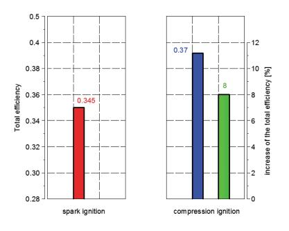
Fig.6. Comparison of the total efficiency the test engine working in spark ignition and compression ignition mode for the speed 2500 rpm
