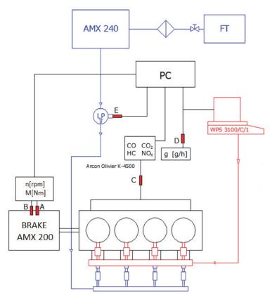
Fig. 1. Scheme of the test stand (symbols: A – meaurement of rotational speed, B – measurement of rotational moment, C – measurement of coefficient of air's surplus, and toxic components of exhaust fumes, D – measurement of mass expense of fuel, for injection of ignition dose, E – measurement of fuel's consumption of fundamental dose
